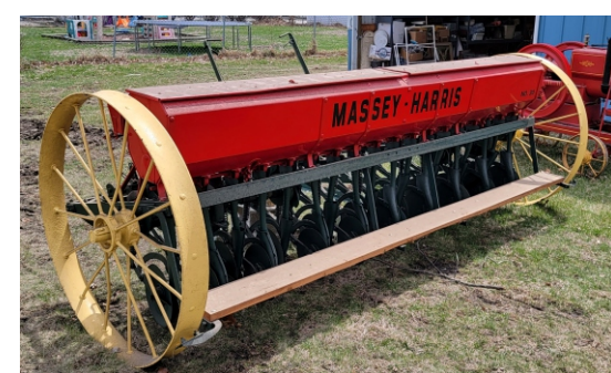
Massey Harris #30 Drill on Steel Grass seed boxes, Restored, Wheel scrapers
