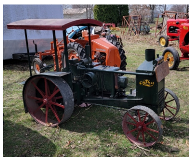
Rumley Oil Pull Tractor Homemade, 3.5 hp International Engine/Transmission
